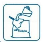
Remove the cap and insert the pre-filter into the SolarBag, fold elastic edge over the SolarBag opening to hold in place. Pour the source water through the pre-filter until the SolarBag is full. Remove the pre-filter and replace the cap.
